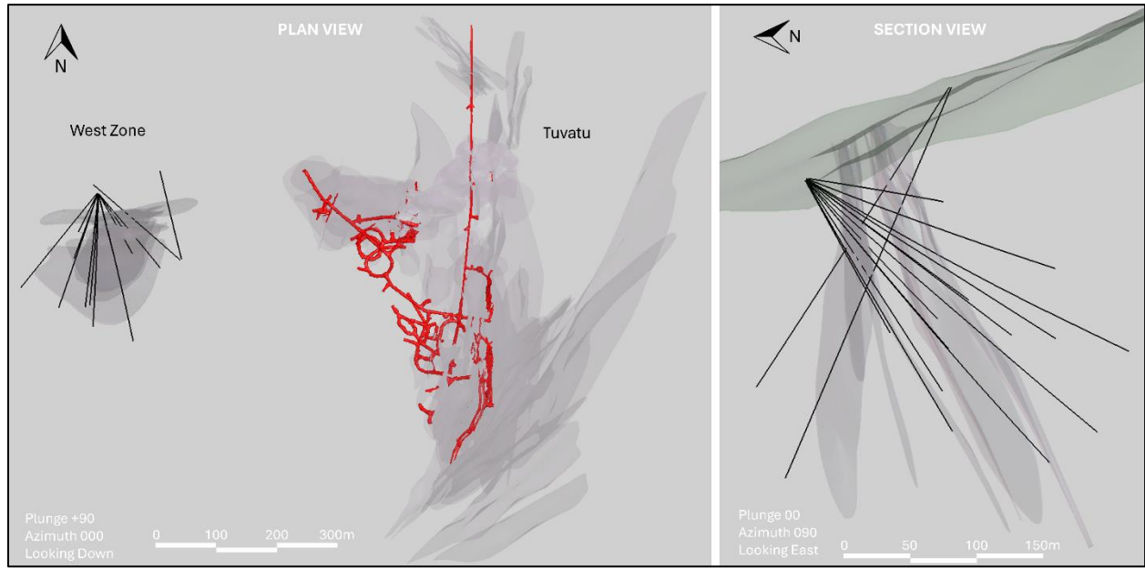
Figure 1. Location of the West Zone drilling reported in this news release. Left image: Plan view of the West Zone drilling in relation to the mineralized lodes shown in grey and Tuvatu underground development shown in red. Right image: Section view of the West Zone drilling looking east.
