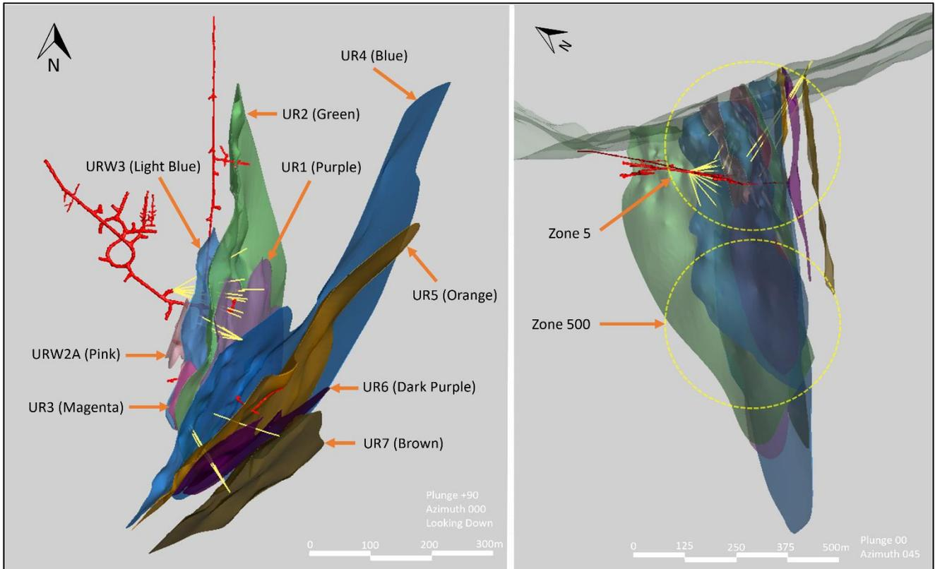
**Figure 2. Main Zone at Tuvatu.** Left image: Plan view of Tuvatu identifying the lodes referenced in this report. Right image: Section view looking approximately northeast, showing the location of Zone 5 and Zone 500 relative to the lodes. Drillholes reported in this news release are shown in yellow for visibility.
