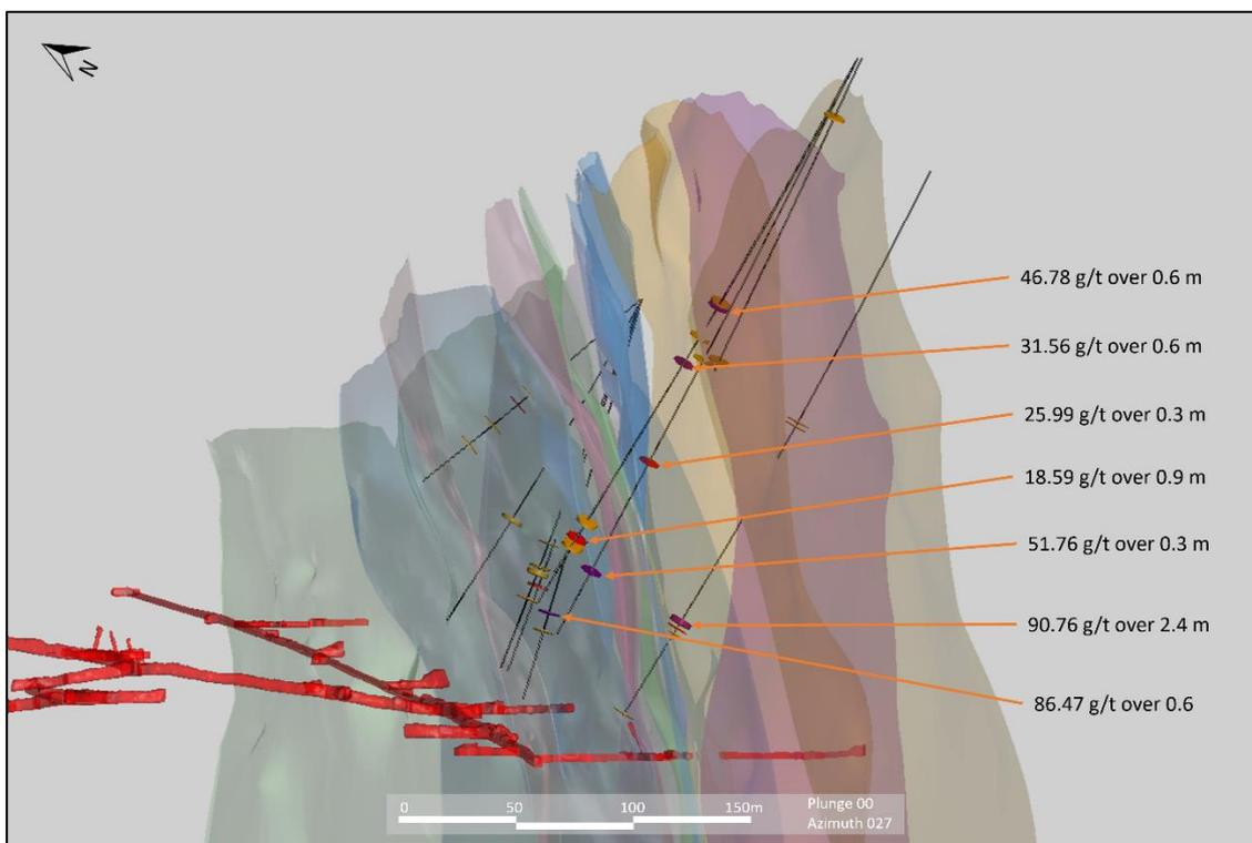
**Figure 4. Location of High-Grade Gold Intercepts from Zone 5 Infill Drilling, 3.0 g/t cutoff.** High-grade gold intervals from Zone 5 infill drillholes reported in this news release. Composite intervals with grades between 3 and 10 g/t gold are shown in orange, intervals with grades between 10 and 30 g/t gold are shown in red, and intervals over 30 g/t gold are shown in purple. Select high-grade intervals are identified. View is looking approximately NNE.
