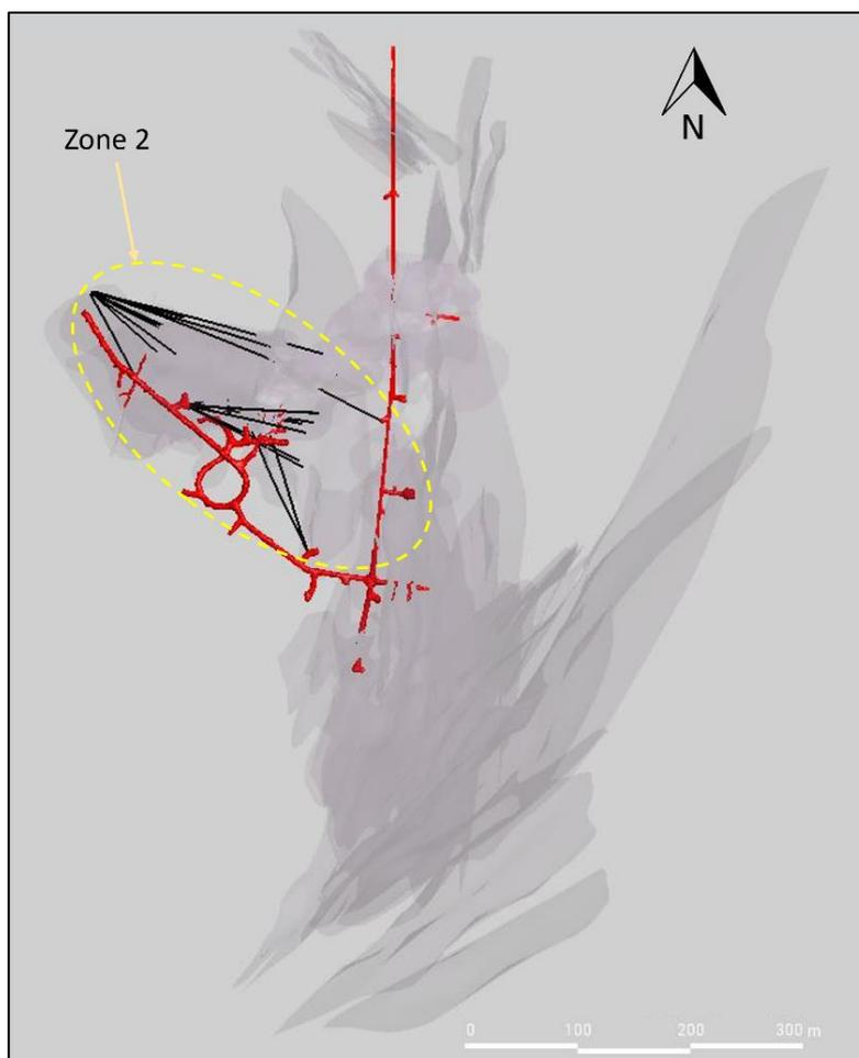
**Figure 1. Location of Zone 2 Grade Control Drillholes.** Left image: Plan view of Tuvalu showing Zone 2 grade control drillholes in relation to the mineralized lodes. Drillholes are shown in black, mineralized lodes in pale grey, and underground developments in red. The yellow dashed circle represents the Zone 2 area of the deposit.
