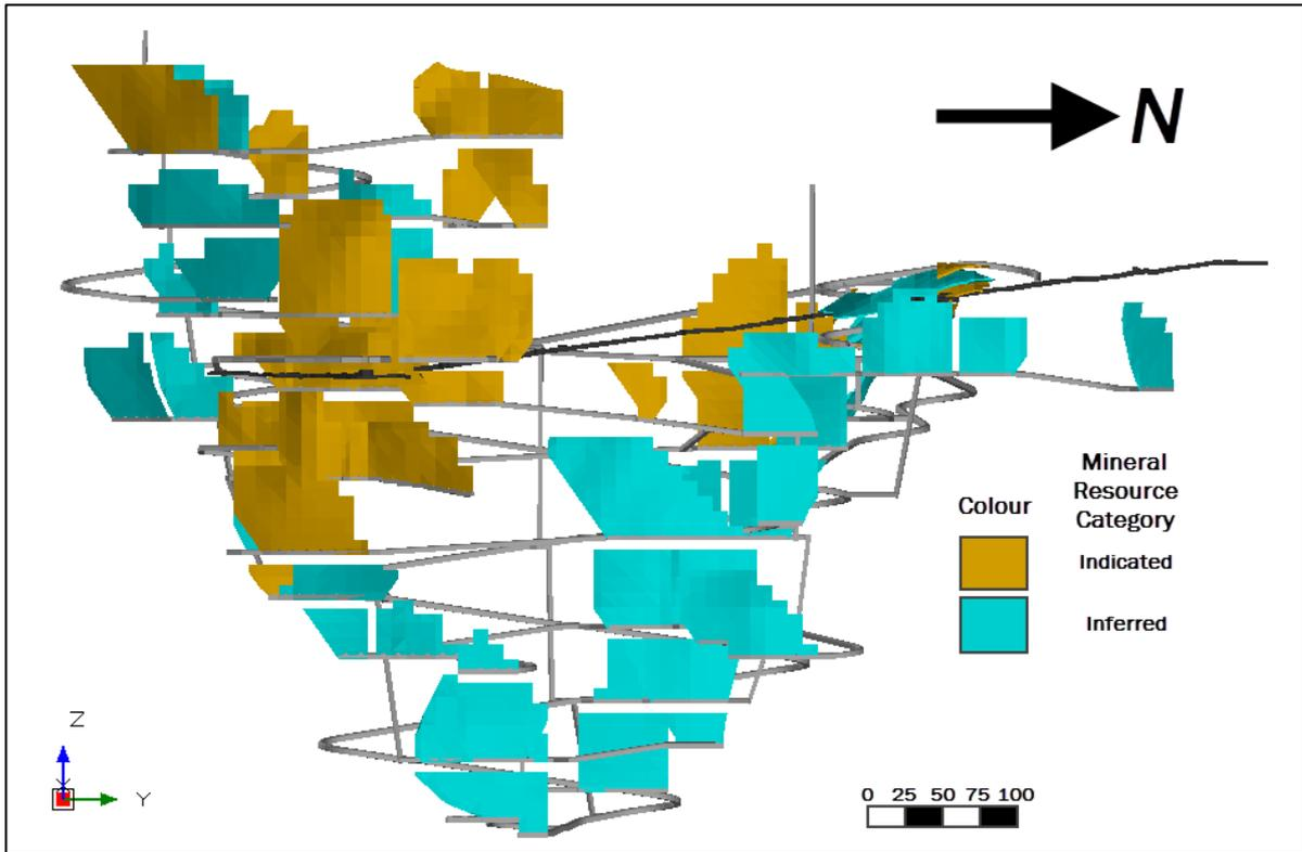
**Figure 16.7 East-west section – Underground conceptual mining blocks**
